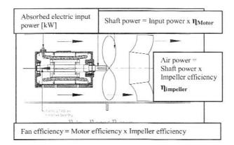
Figure 6: Schematic diagram of an axial fan
