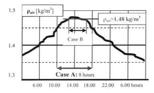
Figure 7: Air density variation at UDL = 3220 mm (Pitis 2006)
