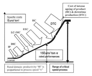
Figure 9: Specific costs evolution function of the process speed for a specific mining process
