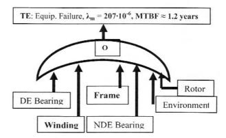
Figure 4: Typical fault tree used for estimation of reliability indicators of an electric motor
