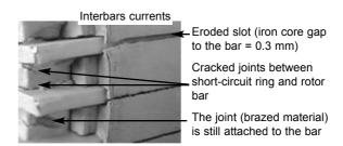
Photo 2: Cracked 220mm 2 joints of a 200 kW rotor
