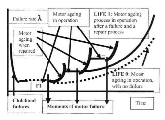
Figure 5: Schematic diagram of failure rates evolution
