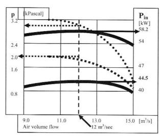
Air pressure 'p' vs. air volume flow (dot lines) Absorbed electric power: Pin (solid lines) Standard  $\rho_{air} = 1.2 \text{ kg/m}^3$  (bottom horizontal) UDL  $\rho_{air} = 1.48 \text{ kg/m}^3$  (top horizontal)
