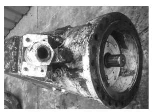
Photo 4: Gathering arm (spinner) motor fitted with MCFR, after 1.8 years working underground
