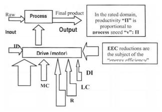
Figure 1: TCO structure of an application (drive) used for a particular mining process
