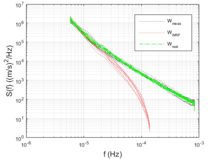
**Figure 7: Power spectral densities  $S(f)$  of measured wind speeds  $w_{meas}$ , for ten masts in South Africa and the corresponding weather model wind speeds  $w_{WRF}$  and real time wind speeds  $w_{real}$  simulated with CorWind.**
