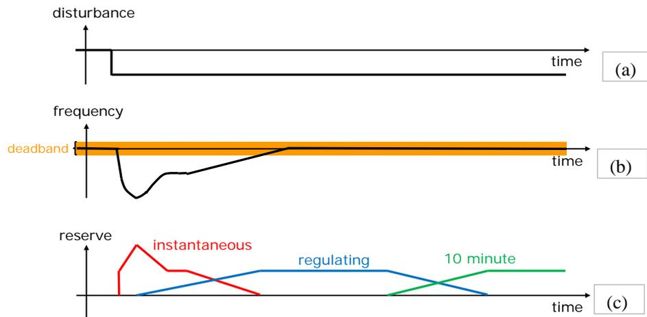
**Figure 12. Illustration of the use of different reserve categories in the case of a contingency disturbance, where (a) is a sudden change in power balance; (b) is the corresponding impact on the system frequency; and (c) is the activation of reserves of different categories.**
