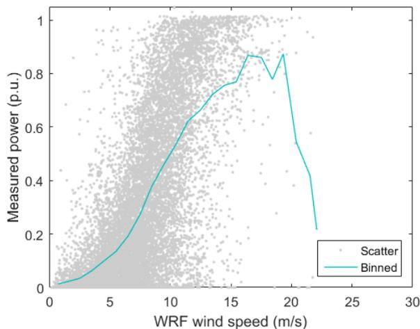
**Figure 3: Power curve estimation using method of binning.**
