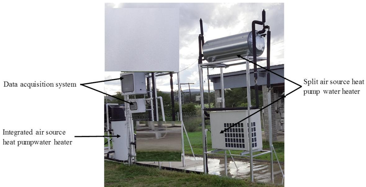
**Figure 1: Experimental set up for the investigation.**
