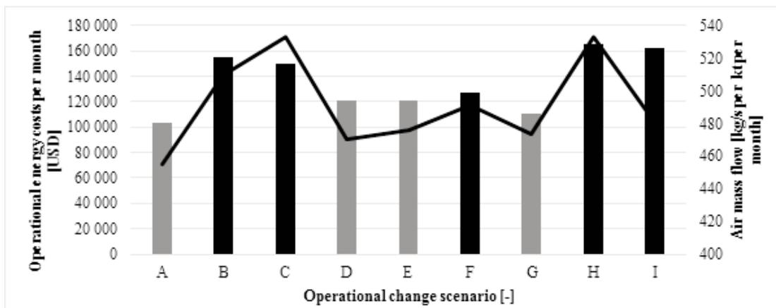
Figure 5: Operational costs per month in US dollars (bar) and total air mass flow rates (line) per operational change scenario.
