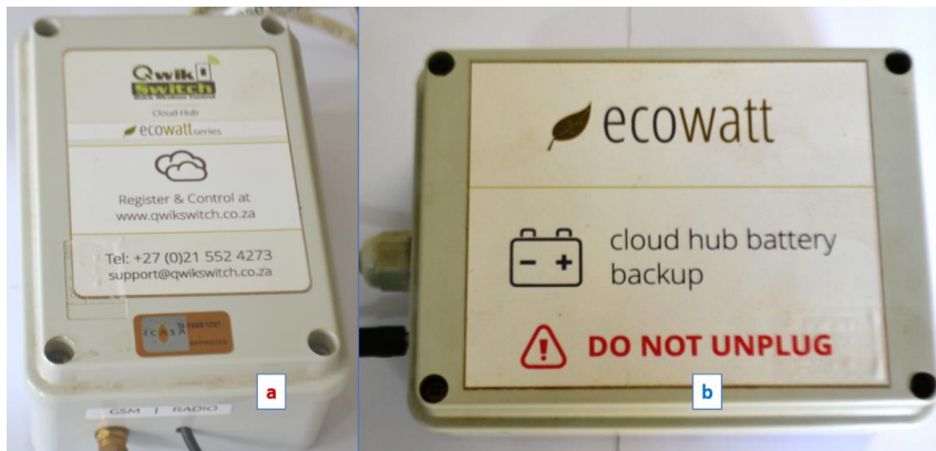
Figure 5: a) Cloud Hub™ data logger, b) Battery back-up.
