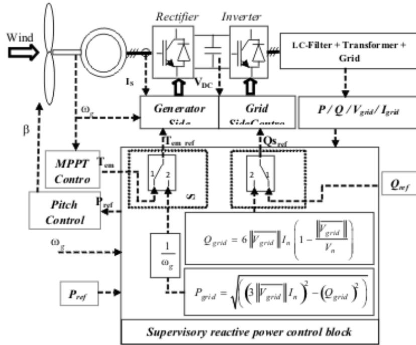
Figure 13: Schematic diagram of the reactive power supervisory
