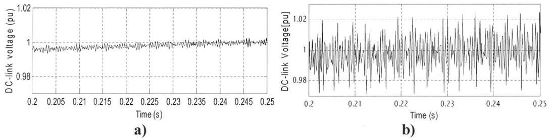
**Figure 9: DC-link voltage: a) VOC techniques b) DPC techniques**
