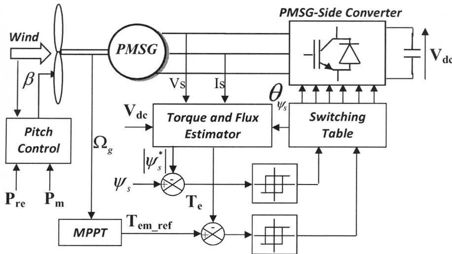
Figure 3: Block diagram of the direct torque control
