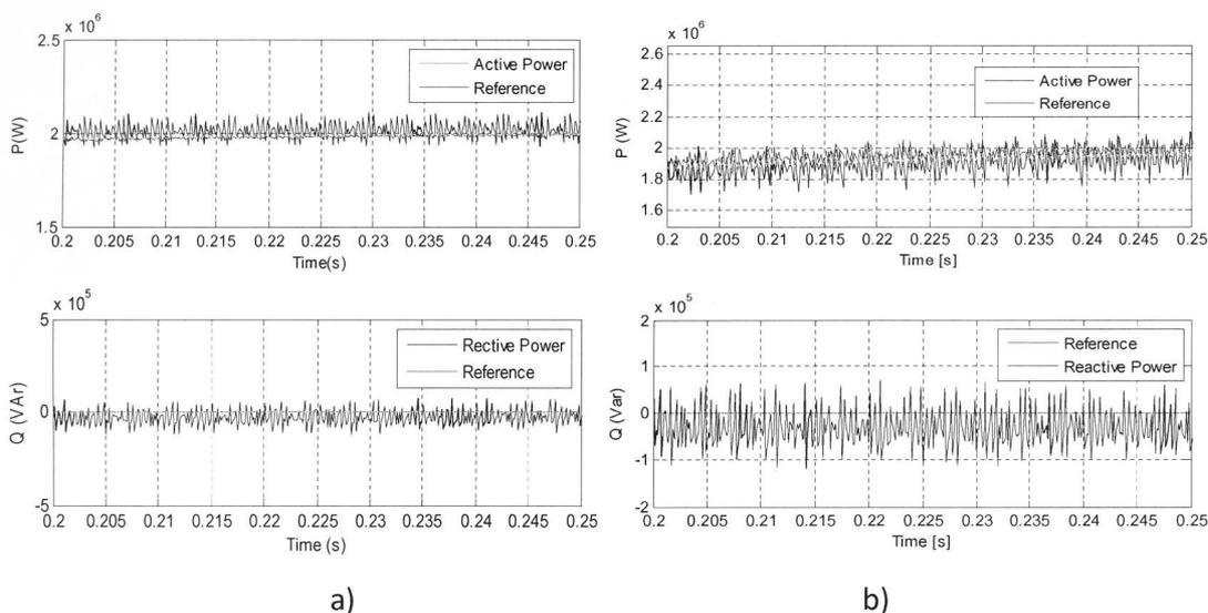
Figure 8: Active and reactive power behaviours: a) VOC techniques b) DPC techniques
