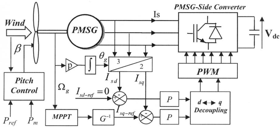
Figure 2: Block diagram of the field oriented control
