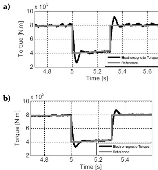
Figure 4: Simulation results versus the time-domain waveforms of the PMSG electromagnetic torque, during a load transient: a) FOC technique; b) DTC technique
