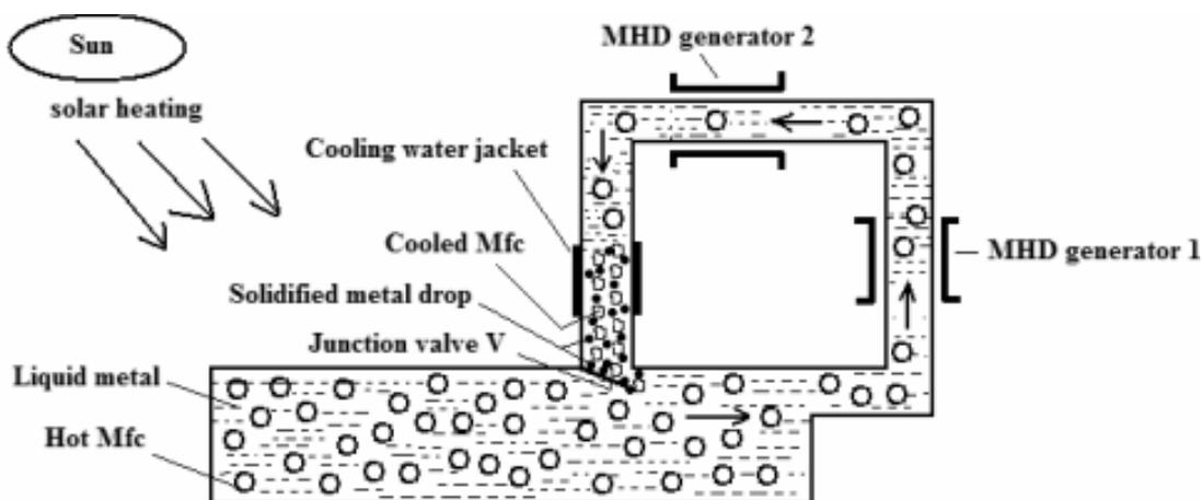
Figure 7: Schematic diagram of a dual cycle LMMHDEC system
