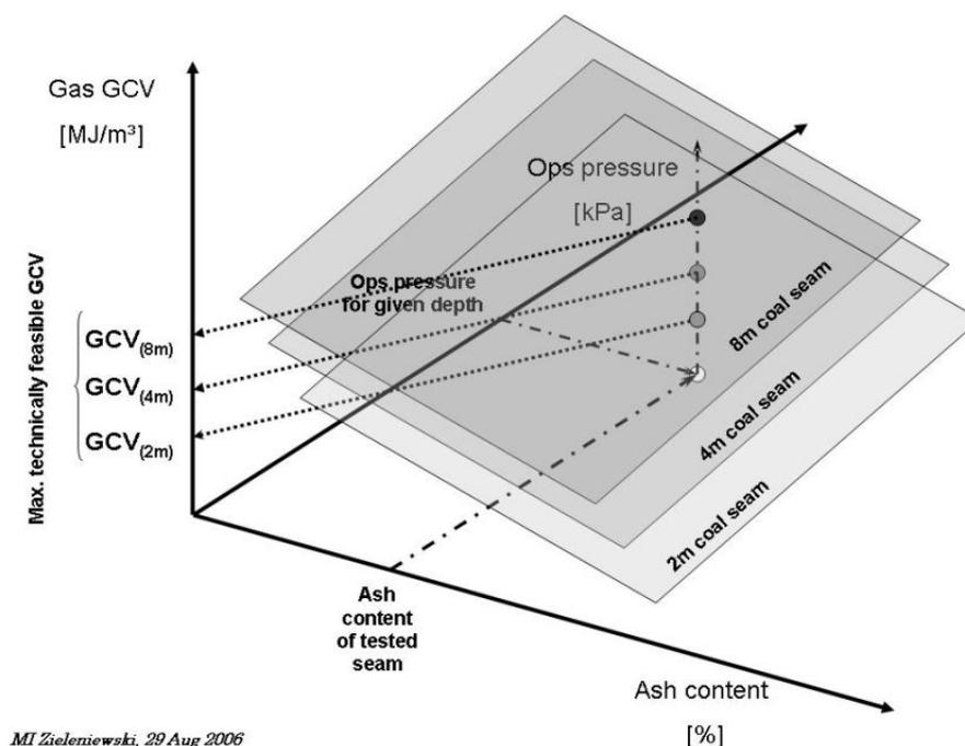
**Figure 3: Relationships of feasibility stage test ( $GCV_{tmx}$  finding)**
