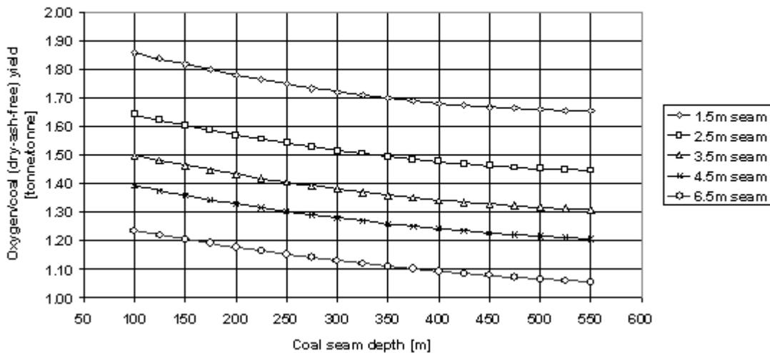
**Figure 4: Expected oxygen/coal (dry-ash-free basis) yield vs coal seam depth and thickness**
