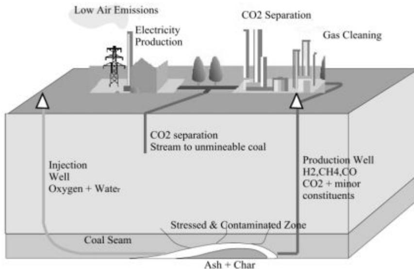
**Figure 1: The main components of a commercial UCG site for power generation**
