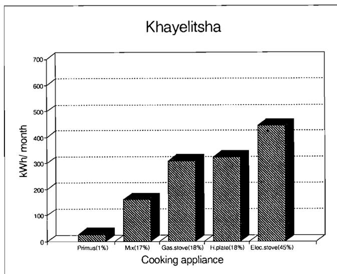
Figure 8a: Total electricity consumption for households in Khayelitsha using various cooking appliances
