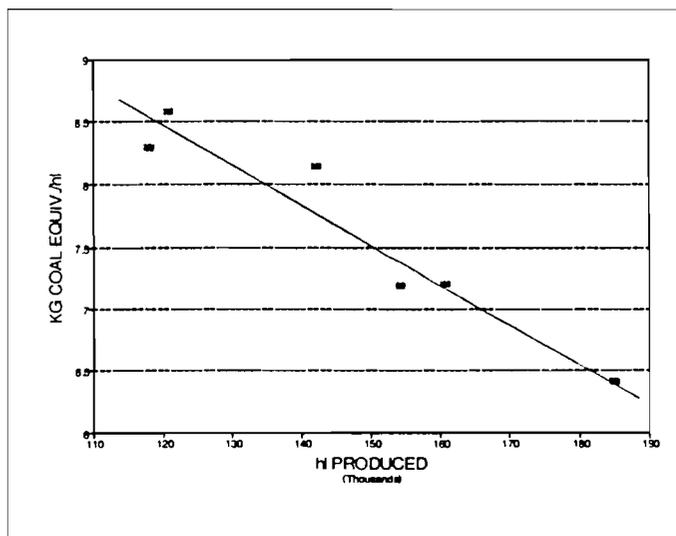
Figure 3: Specific coal equivalent requirements for various monthly quantities of beer produced
