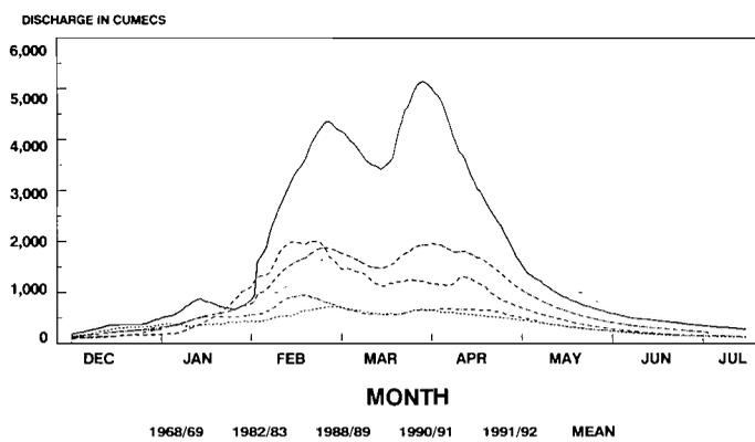
Figure 9: Various (flow) hydrographs of the Zambezi at Chavuma
