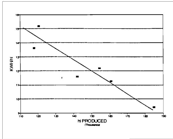
Figure 4: Specific electricity requirements for various monthly quantities of beer produced
