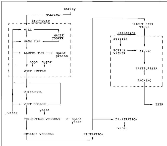
Figure 1: Diagram of the brewing process
