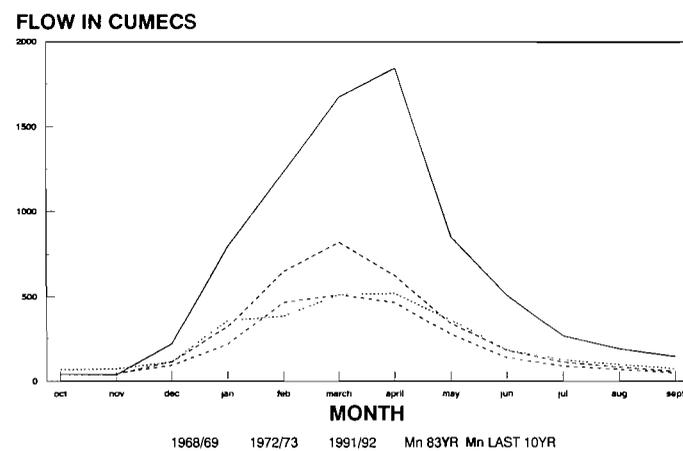
Figure 10: Various (water-level) hydrographs of the Zambezi at Lukulu
