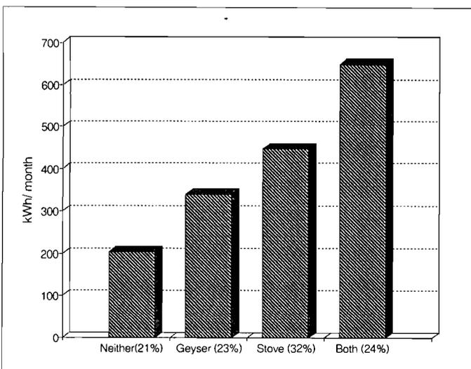
Figure 9: Total electricity consumption for households using various stoves and/or geysers
