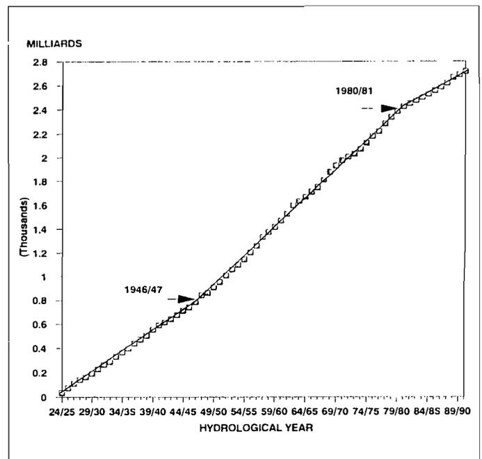
Figure 4: Cumulative run-off (mass) curve of the Zambezi at Livingstone/Victoria Falls
