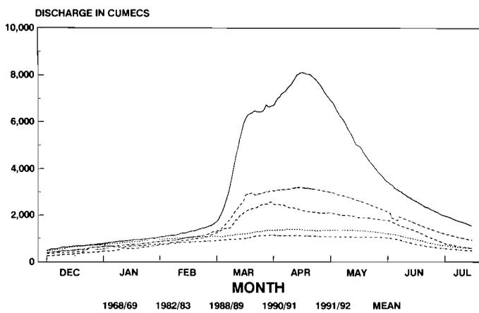
Figure 8: Various (flow) hydrographs of the Zambezi at Victoria Falls
