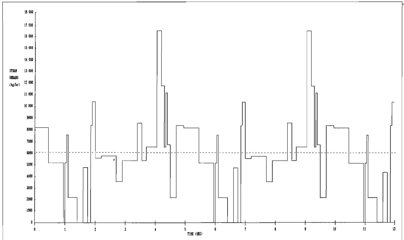
Figure 5: Steam demand profile for the brewhouses operating on a five-hour cycle
