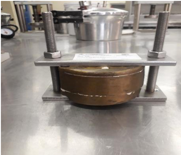
Figure 2: RS flask closure method
