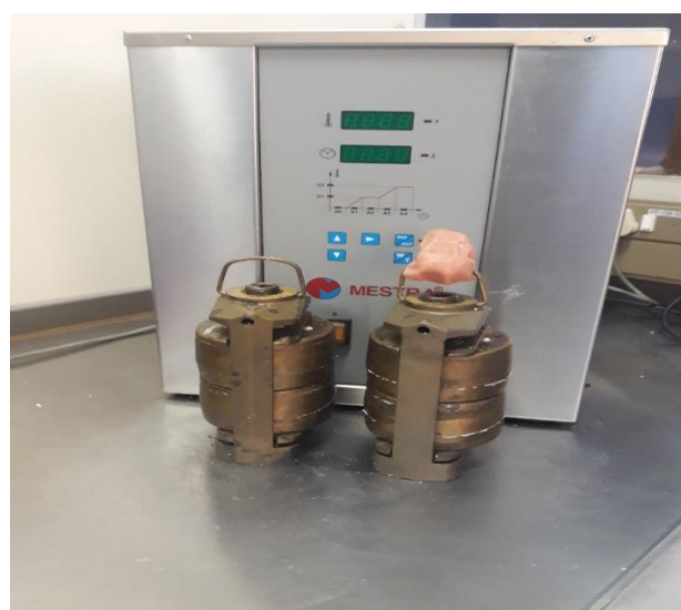
Figure 1: Conventional flask closure method
