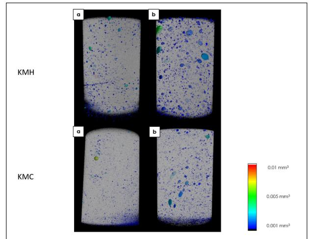
**Figure 4.** Micro-CT 3-D reconstructed images of KMH and KMC. Panel a) indicates the representative material samples with the smallest volume of voids and panel b) the specimen with the largest volume of voids.
