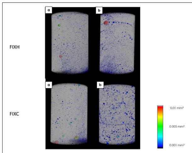
**Figure 2.** Micro-CT 3-D reconstructed images of FIXH and FIXC. Panel a) indicates the representative material samples with the smallest volume of voids and panel b) the specimen with the largest volume of voids.
