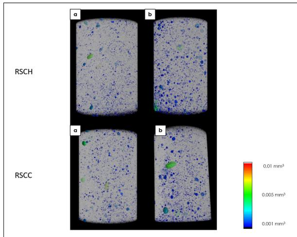
**Figure 1.** Micro-CT 3-D reconstructed images of RSCH and RSCC. Panel a) indicates the representative material samples with the smallest volume of voids and panel b) the specimen with the largest volume of voids.
