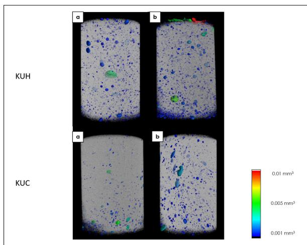
**Figure 3.** Micro-CT 3-D reconstructed images of KUH and KUC. Panel a) indicates the representative material samples with the smallest volume of voids and panel b) the specimen with the largest volume of voids.
