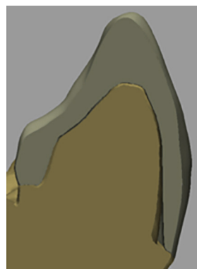
Figure 6. Crown preparation with undercuts and resulting overmilled restoration (Illustration courtesy of Sirona)
