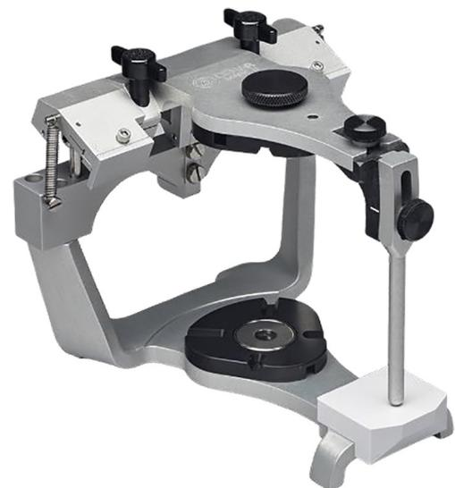
Fig. 7. An arcon articulator: the 'condyle is on the lower member and the 'fossa' on the upper member.
