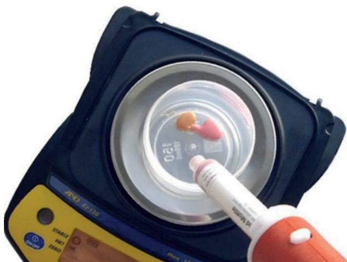
Figures 7 & 8: Recipe weight of colouring system and addition of Platinum Silicon Part A and B according to recipe 15
