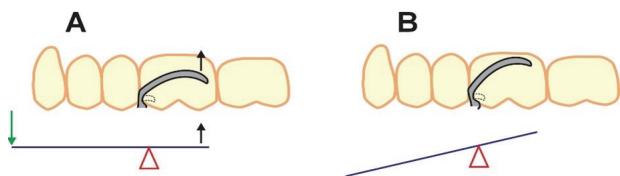
Figure 18 A: If the denture rotates downwards anteriorly and a clasp assembly has a mesial rest with the clasp engaging the distal undercut, a Class I lever is created with the mesial rest as fulcrum. B: this means that the clasp now moves in the wrong direction and does not engage the bulge of the tooth and so provides no retention.
