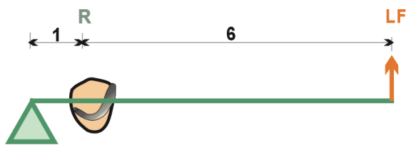
Figure 17. The beam of a mandibular distal extension base as a Class II lever. The effort arm is from the lifting force (LF) to the fulcrum, the resistance arm R is from the clasp to the fulcrum.
