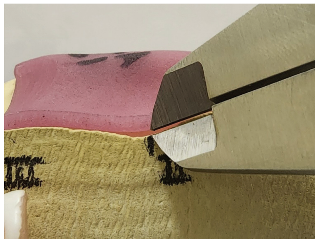
Figure 4: Measuring the gap distance between the baseplate and the cast at position II.
