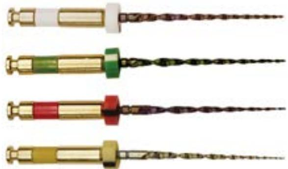
Figure 10. EdgeOne Fire (EdgeEndo), Small (Yellow 20/06), Primary (Red 25/06), Medium (Green 35/045) and Large (White 45/03) .
