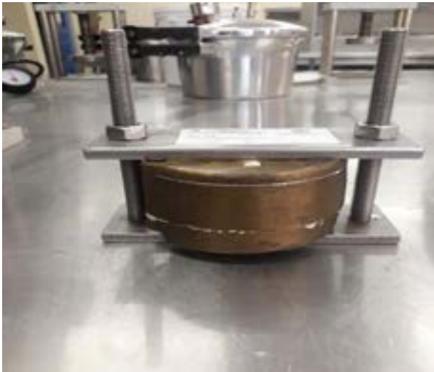
Figure 2: RS flask closure method
