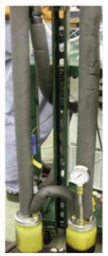
Figure A3: Bio-oil condensers and containers
