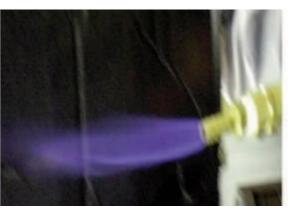
Figure A5: Combustibility test of NCG
