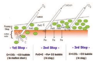
Figure 3: Mechanism of foaming slag creation
