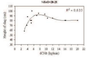
Figure 9: Variation of carbon injection rate with slag height Source: Aminorroaya and Edris (2002)
