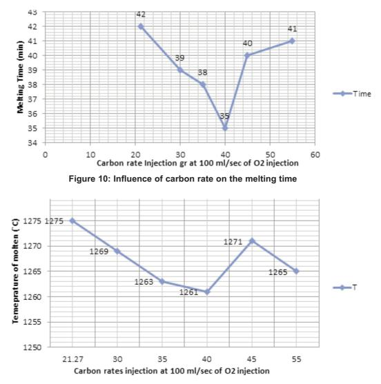
Figure 11: Influence of the carbon rate injection on the temperature of the melt
