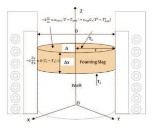
Figure 17: Sketch of the induction furnace
