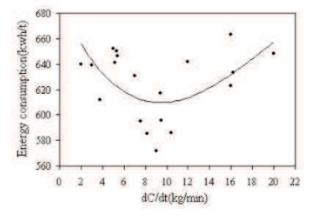
Figure 14: Variations of carbon injection rate with electrical energy consumption Source: Aminorroaya and Edris (2002)
