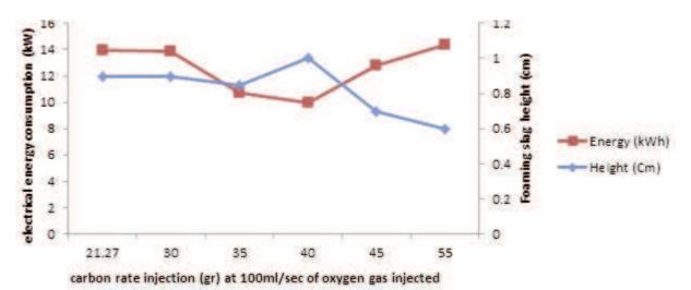
Figure 13: Relationship between the electrical energy consumption and the foaming slag height (cm)
