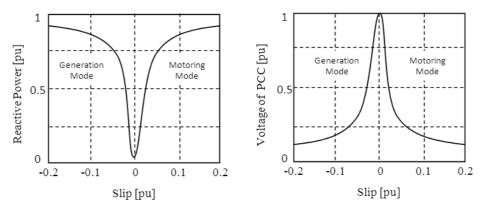
Figure 1: (a) Reactive power response for varying slip (b) Voltage response for varying slip
