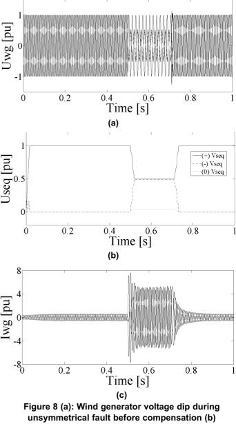
unsymmetrical fault before compensation (b) sequence components during dip (c) Current overshoot during dip
