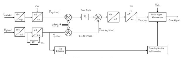
Figure 4: Vector controller scheme
