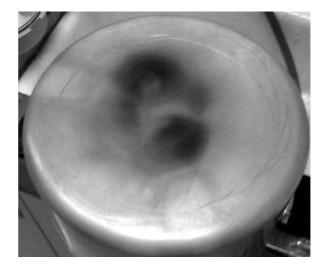
Figure 3: Base of pot after a single cooking test
