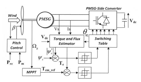
Figure 3: Block diagram of the direct torque control
