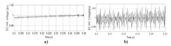
Figure 9: DC-link voltage: a) VOC techniques b) DPC techniques
