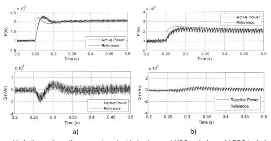
Figure 11: Active and reactive power transient behaviours: a) VOC techniques b) DPC techniques
