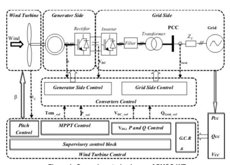
Figure 1: General control scheme of PMSG-WT
