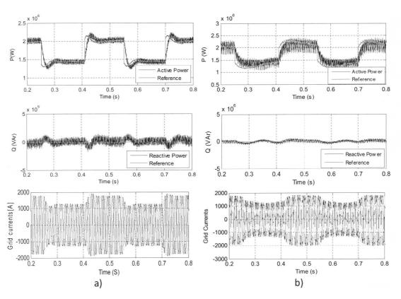
Figure 10: Instantaneous response during active and reactive power reference steps: a) VOC techniques b) DPC techniques
