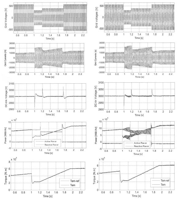
Figure 14: Wind turbine behaviour during a asymmetrical fault (type A), with the VOC techniques
