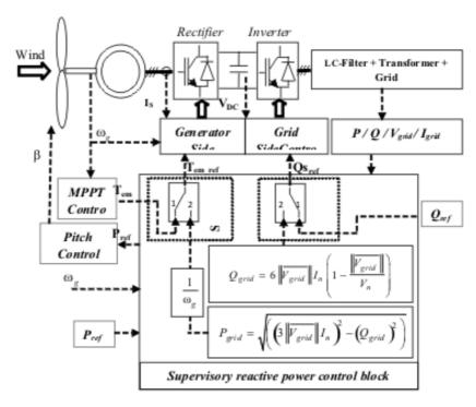
Figure 13: Schematic diagram of the reactive power supervisory
