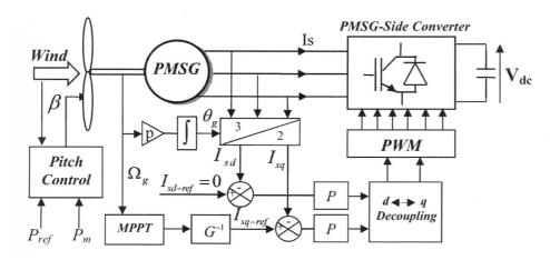
Figure 2: Block diagram of the field oriented control
