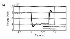
Figure 4: Simulation results versus the timedomain waveforms of the PMSG electromagnetic torque, during a load transient: a) FOC technique; b) DTC technique
