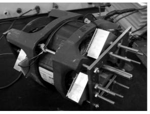
Figure 5: Photo of the single-phase asynchronous machine with the TECM housing structure
