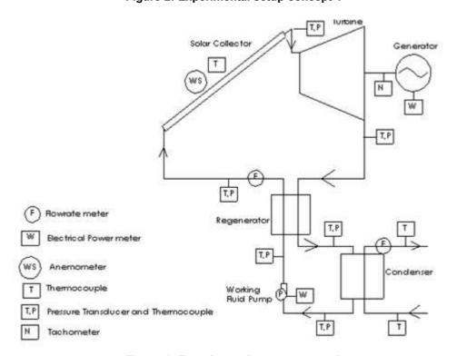
Figure 3: Experimental setup concept 2
