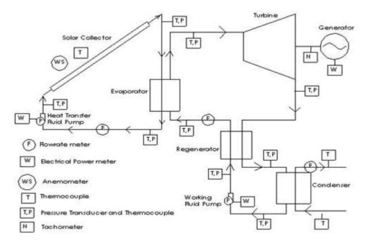
Figure 2: Experimental setup concept 1
