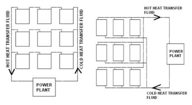
Figure 4: Two layouts options for 500 Wp solar field (requires 9 solar collectors with two layout options)
