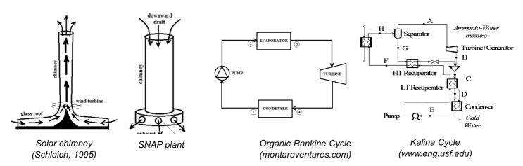
Figure 1: Examples of low temperature solar thermal energy technologies
