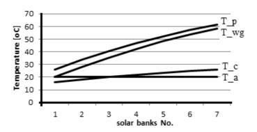
Figure 12: Temperature profile along solar banks; 180collector model
