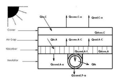
Figure 8: One pipe solar collector model
