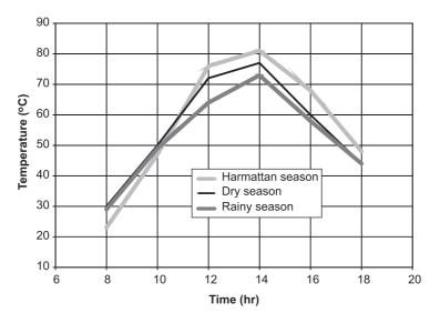
Figure 1: Hourly temperature profile of the NCERD solar water heater for various seasons
