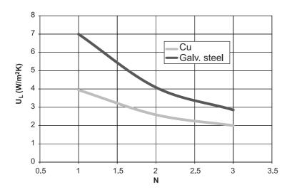
Figure 2: Variation of top-loss coefficient with number of glazing covers, N
