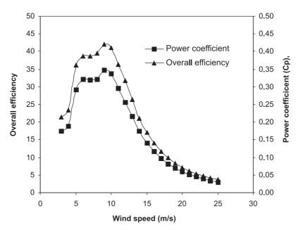
Figure 4: Power coefficient and overall efficiency of 1 MW capacity wind turbine
