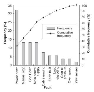
Figure 3: Fault analysis by using the Pareato Chart for the wind farm, Motha
