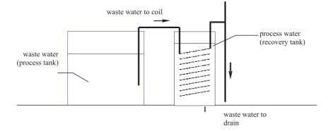
Figure 5: Coil heat exchanger for heat recovery from waste water to process water
