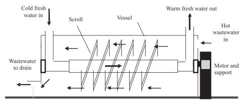
Figure 3: Spiral or rotary heat exchanger
