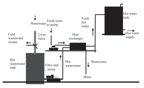
Figure 1: Centralised waste water heat recovery
