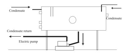
Figure 2: Pump and condensate receiver
