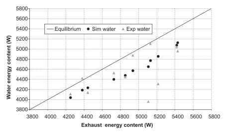
Figure 9: Heat exchanger experimental and simulated energy balance
