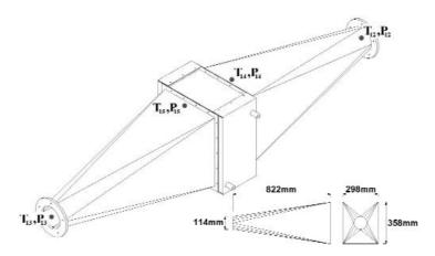
Figure 3: Measurements taken on the exhaust inlet ducting
