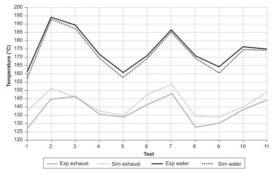
Figure 8: Actual and simulated outlet temperatures
