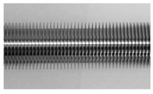
Figure 1: NC-machined finned tube
