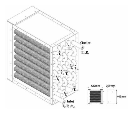
Figure 2: Measurements taken on the heat exchanger
