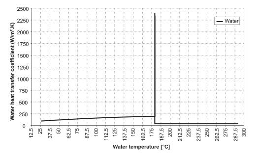
Figure 12: Water heat transfer coefficient vs. temperature
