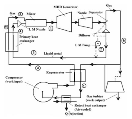
1, 2, 3, 4 > Liquid metal loop, and a, b, c, d, e > Gas/ Vapour loop
