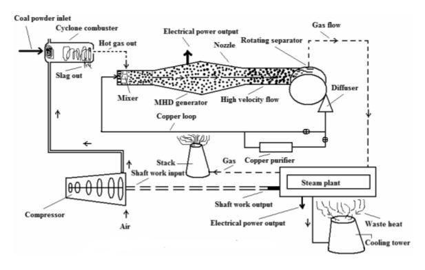
Figure 5: A schematic diagram of an open cycle LMMHDEC system
