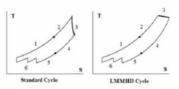
Figure 1: Standard Brayton Cycle compared with MHD Brayton Cycle
