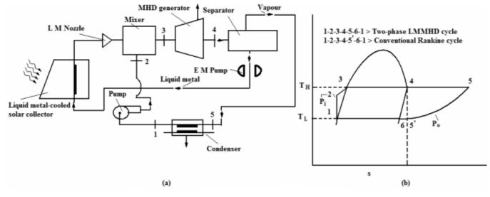
Figure 4 (a & b): Schematic diagram of solar-assisted LMMHD Rankine cycle with liquid metal cooled collector
