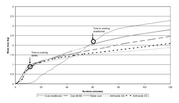
Figure 5: Mass loss versus time for the four Basa njengo Magogo fires and the bottom-up ignited coal fire
