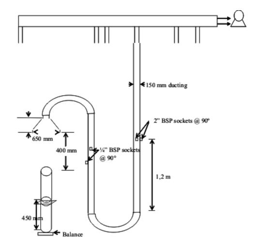
Figure 1: Setup for the low smoke fuel testing
