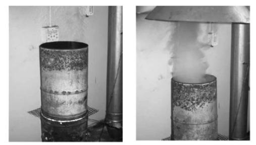
Figure 6: Comparative smoke emissions from the Basa njengo Magogo fire (left) and a fire ignited with the bottom-up method (right), using traditional D-grade coal
