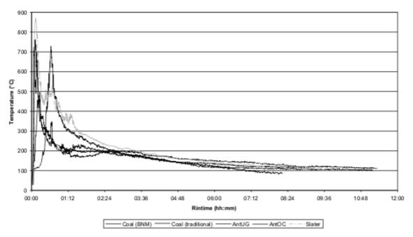
Figure 4: Temperature variation during the four Basa njengo Magogo fires and the bottom-up ignited coal fire. The low values between 30 and 40 minutes coincide with the water boiling part of the experiment, when the temperature sensor was removed
