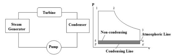
Figure 1: Key components of a thermal power plant working on a Rankine Cycle
