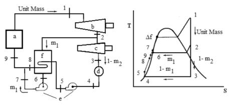
(a)- Steam Generator, (b)- High Pressure Turbine, (c)- Low Pressure Turbine, (d)- Condenser (e)- Pump, (f)- Closed FWH
