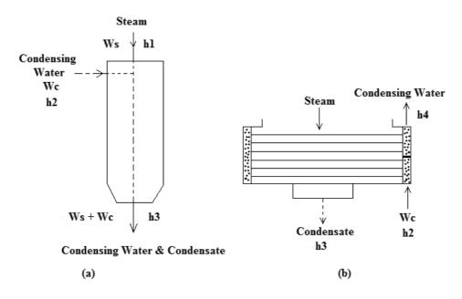
Figure 3: Energy exchange in a condenser
