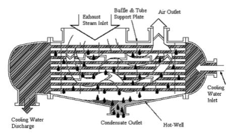
Figure 6: Single pass condenser
