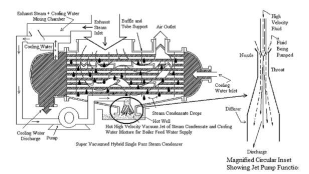
Figure 8: A super vacuum hybrid pass steam condenser
