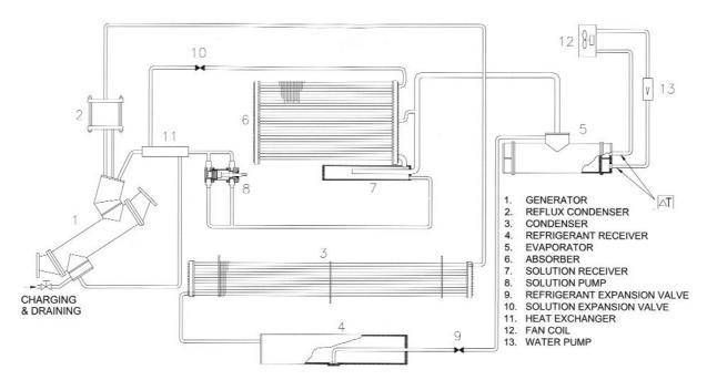
Figure 3: Schematic diagram of the assembly of the absorption air-conditioning system
