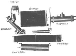
Figure 2: Components of the car airconditioning plant
