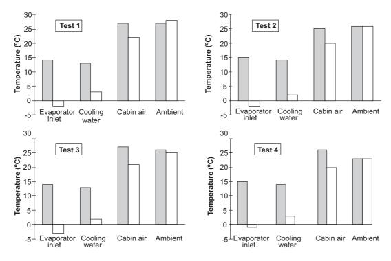
Figure 5: The shaded and the clear areas indicate the temperature conditions before and during the road-tests respectively
