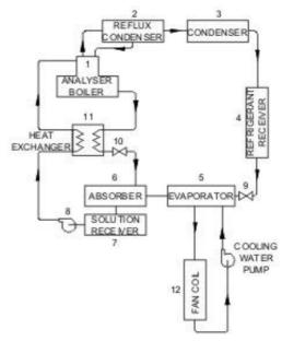
Figure 1: Schematic arrangement of the absorption system
