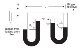
Figure 3: Set-up of the experiment
