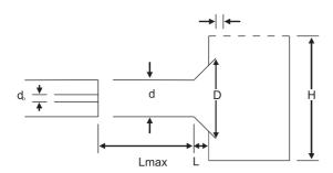
Figure 2: Schematic diagram of the burner
