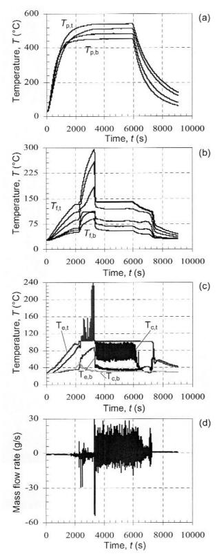
Figure 4: (a) Heating plate temperatures (b) Fin temperatures (c) Working fluid temperatures (d) Mass flow rate
