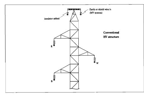
Figure 1: Typical earth wire tower configuration
