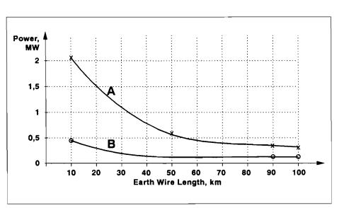
Figure 9: Power transfer capacities of earth wires
