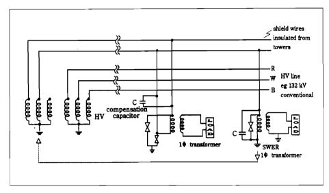
Figure 2: Single-phase (balanced) and SWER schemes
