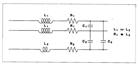
Figure 4: Three-phase scheme phase impedances
