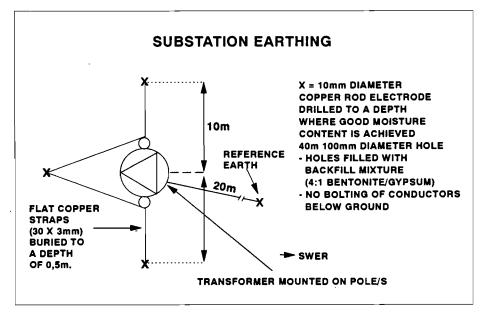
Figure 7: Earthing option for ensuring low earth resistance in high resistivity soils
