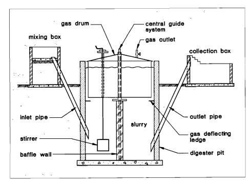
Figure 1: Sketch of the biogas plant installed at the Mathabela homestead
