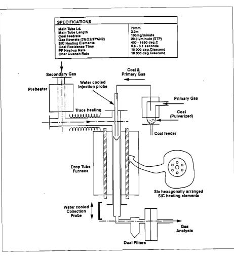
Figure 1: Eskom's drop tube furnace
