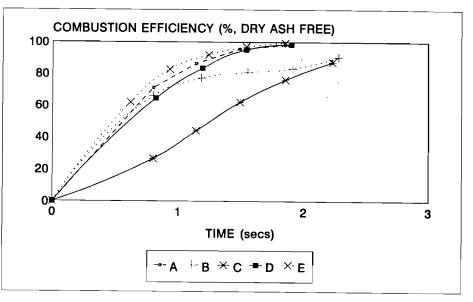
Figure 2: Combustion efficiency vs time (1 400 deg.C,  $3\% O_2$ )
