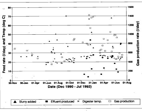
Figure 2: Recorded feeding rate, digester temperature and gas production rate
