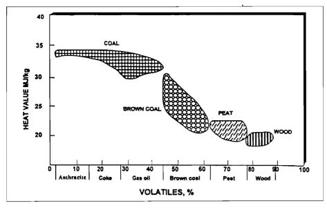
Figure 1: Peat relative to wood and other fossil fuels in terms of its heat value and volatile content
