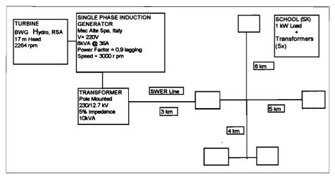
Figure 10: Basic electrical configuration of the scheme
