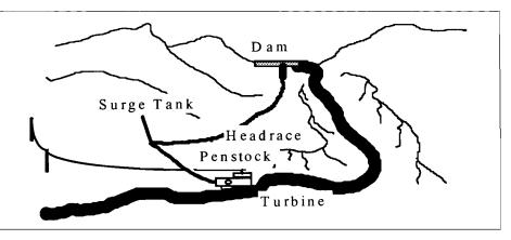
Figure 3: Components of the Ntonyelana micro hydro scheme
