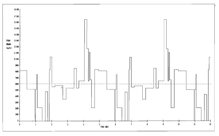
Figure 5: Steam demand profile for the brewhouses operating on a five-hour cycle
