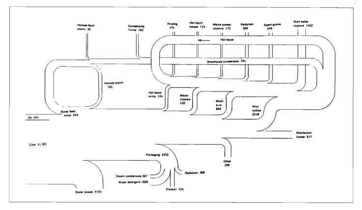
Figure 6: Sankey diagram for fuel and steam
