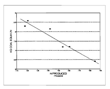
Figure 3: Specific coal equivalent requirements for various monthly quantities of beer produced
