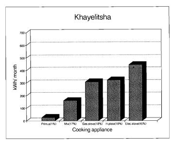
Figure 8a: Total electricity consumption for households in Khayelitsdha using various cooking appliances
