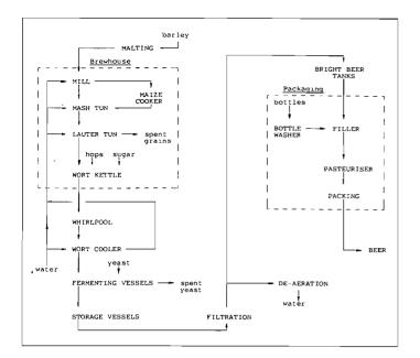
Figure 1: Diagram of the brewing process
