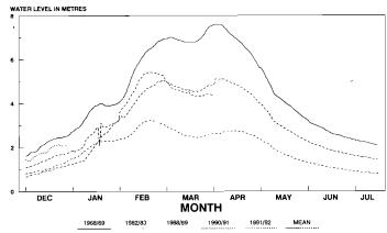
Figure 11: Various (flow) hydrographs of the Kafue at Itezhi-Tezhi
