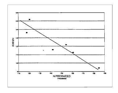
Figure 4: Specific electricity requirements for various monthly quantities of beer produced
