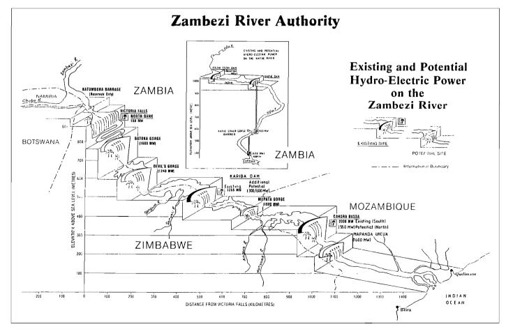
Figure 2: Existing and potential hydroelectric power sites on the Zambezi River
