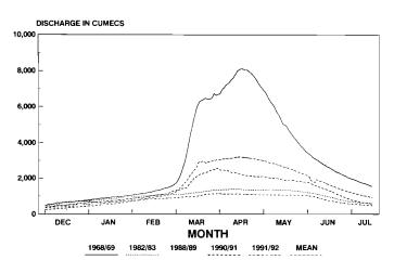
Figure 8: Various (flow) hydrographs of the Zambezi at Victoria Falls
