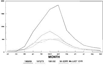
Figure 10: Various (water-level) hydrographs of the Zambezi at Lukulu
