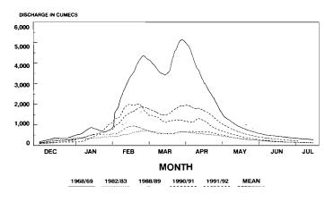
Figure 9: Various (flow) hydrographs of the Zambezi at Chavuma
