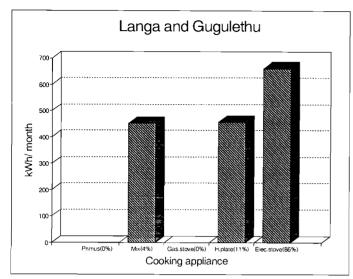
Figure 8b: Total electricity consumption for households in Langa and Gugulethu using various appliances
